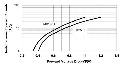
Fig.3-Typical Instantaneous Forward Voltage Characteristics
